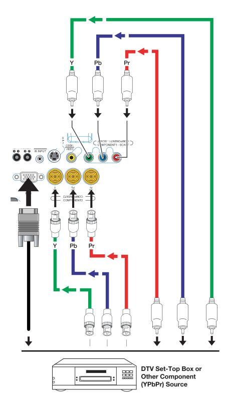
Figure 3-9. Component Video Connections
