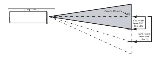
Note: This is a general example of lens shift. Lenses vary in their shift capabilities. No particular lens or projector is used in this example.
