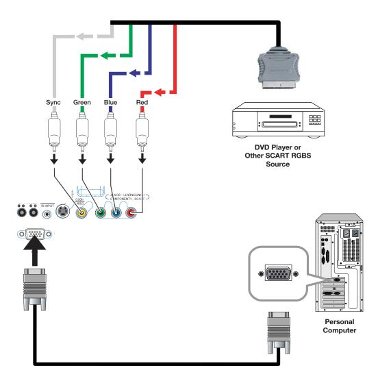
Figure 3-8. RGB Connections
